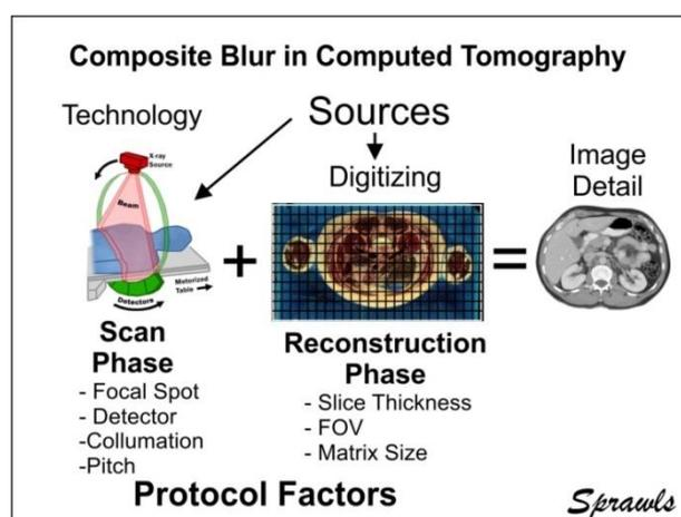
Figure 4. The visibility of anatomical detail in an image is limited by the composite blur from both the equipment design characteristics and the formation of the image in a digital format.
