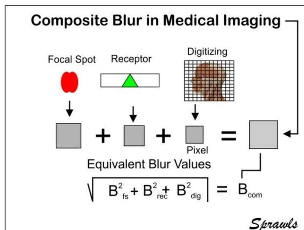
Figure 5. Sources of blur: focal spot ( $B_{fs}$ ), receptor ( $B_{rec}$ ), and digitizing ( $B_{dig}$ ) that combine to form the total or composite blur ( $B_{com}$ ) within an image.
